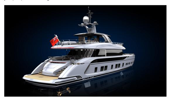
The yacht is powered by two MAN Diesel engines generating near 1700-bhp each. This power is then supplemented by two 45Kw generators which allows this thing to reach speeds up to 21 knots with a range of 6,296 km.
