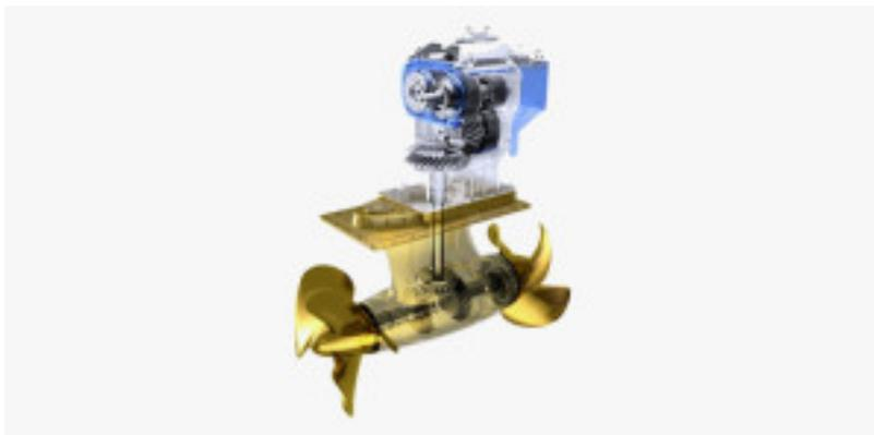
Aligned horizontally, Fortjes pods are supposedly much more efficient than any system using shafts and propellers. Their positioning outside the hull also means greatly reduced noise and vibration levels, as well as lower emissions. The pods use counter-rotating propellers linked via a compact gearbox to the main engines, reducing engine room space requirements by nearly 18%, which means more accommodation. [Fortjes pods](#) are built in Germany.
